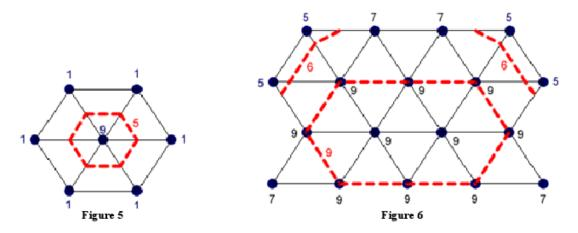
The policy of the ACM is to approximate the actual terrain by a set of triangles constructed by connecting each elevation measurement to its nearest neighbors by straight line segments. Each of these triangles is then treated as a planar surface, where the plane is determined by the coordinates, including elevation, of the vertices. If the triangles are projected onto the zero-elevation plane, they form a set of equilateral triangles.
