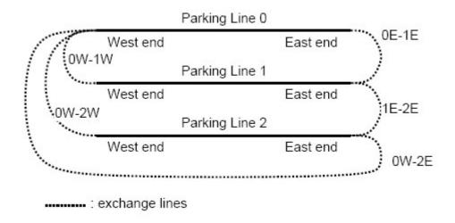
Figure 7: Parking lines and exchange lines
